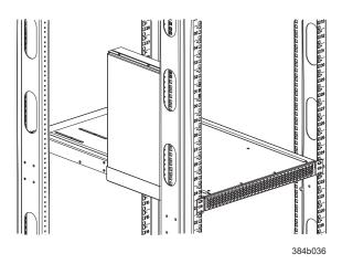
Figure 9. Air duct installed into side slot in shelf
